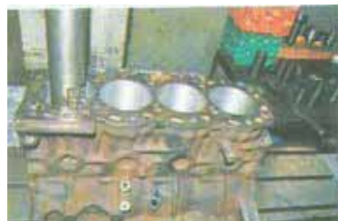
Borind of Block after Resleeving
