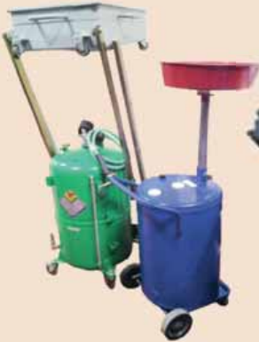
Oil Drain Units
